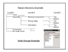
Repair code analysis shows how often Repair Codes or group of codes (for example Assembly/SMD/Top\_Side) has been used. The ordered list shows individual and cumulative percentages.
